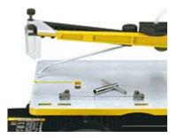
**Patented saw blade holders with high clamping force** ensure true alignment of the saw blades. Recesses in the table surface serve as guide line in assembly to define position and distance of the saw blade holders.
